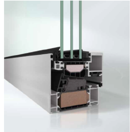
AWS 90 BS.SI+ optimized U_f = 1,0 \text{ W/m}^2\text{K} (99 mm)
